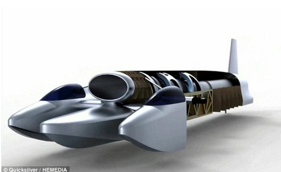
*Diagram showing the major structural features of the centre fuselage, the engine and intake and exhaust layout, and the nose sections only of the two sponsons. Each sponson has a cockpit for pilot (nearest) and engineer (furthest).*
