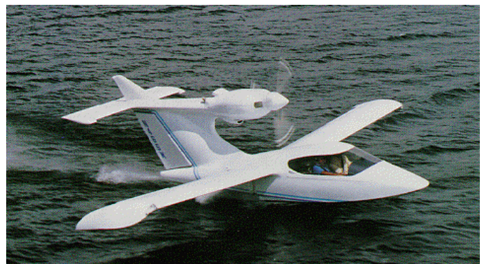
Fig. 16 - Seaplane with Contoured Hull (e.g. Seawind)
