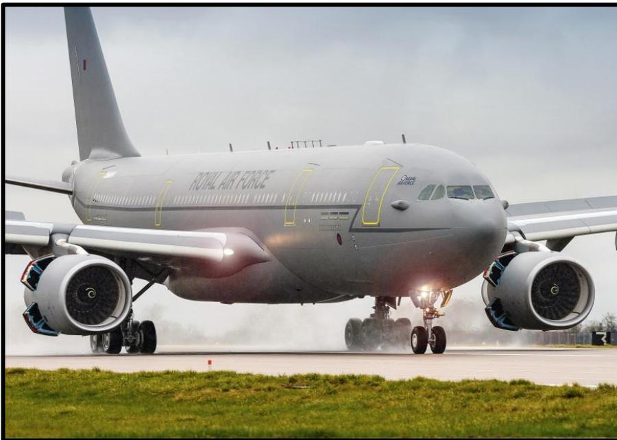
*The Airbus A330-200 'Voyager' is delivered as a standard 291-seat airliner, is then converted to a multi-role configuration, and put into service as an MRCOA (military registered civil owned aircraft )*
