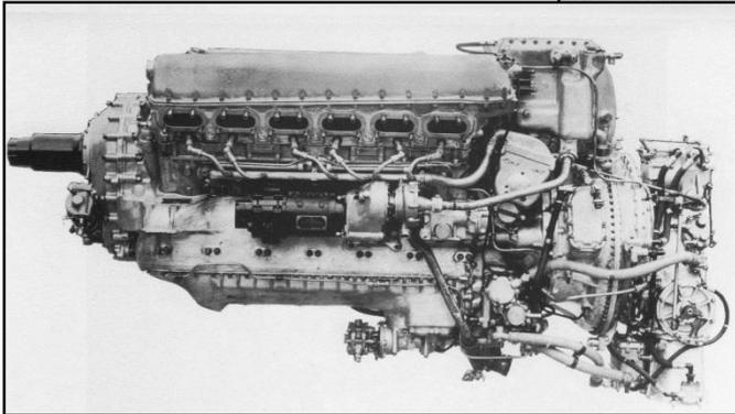
The Merlin 66, was widely used by the RAF from 1942, especially in Spitfire IIX and IX, and provided 1,720HP
