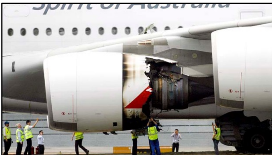
The Rolls-Royce Trent which disintegrated on a Qantas A380 and led to an emergency landing at Singapore (November 2010)
