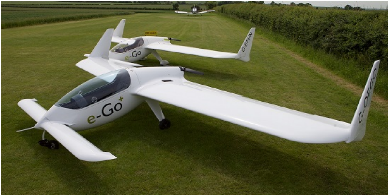
The aircraft in the foreground is the second example built, and the prototype in the background shows the modified wing-tip fin that will be adopted for production.
