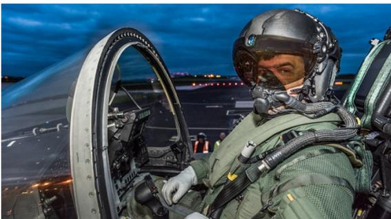
This HMD system was a combination of the visor projected optical system developed for Viper with the modular aircrew helmet from Crusader. It provides today's Typhoon aircrew with a dedicated high capability HMD and was the first high speed ejection cleared binocular HMD to enter service. It was developed by GEC Marconi Avionics in Rochester and Edinburgh who, following the merger with British
