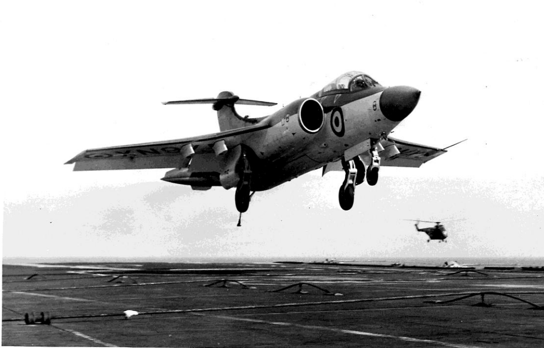
First deck landing trials of the Blackburn Buccaneer II on board HMS Ark Royal – note deployed airbrake
