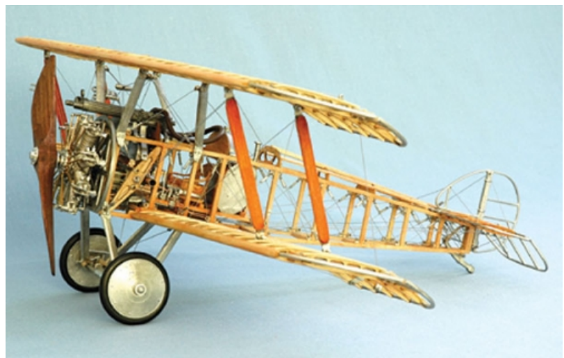
This model of a Sopwith Camel shows the proximity of (from front to back) of engine, armament, cockpit and fuel tank – all are in the forward part of the fuselage.
