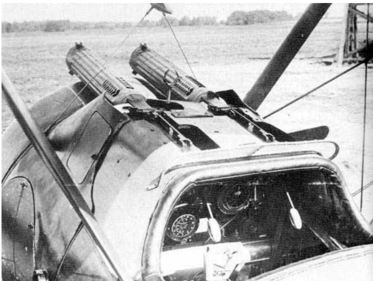
The 'hump' on the Sopwith Camel that neatly integrated the gun controls into the cockpit.
