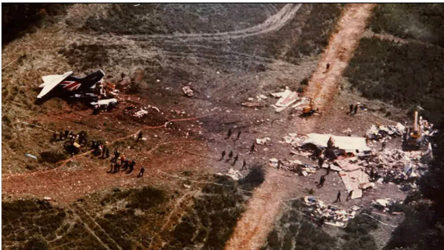
Trident – Staines, near Heathrow 26 June 1972. On departure the aircraft entered a deep stall and crashed in open ground soon after departure. There were no survivors of 118 people on board. Unacceptable cockpit operational procedures caused the loss of control.
