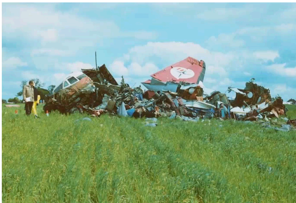
Avro 748 – Nailstone, Leics. 26 June 1981. Separation of aft cabin door, surprisingly occurring during descent, caused the door to become impaled on tailplane leading-edge. This caused sudden migration of stagnation point of flow over tailplane as wing lift coefficient increased during deceleration. This in turn caused dramatic pitch trim change and reversal of pitch control forces at the control column. The net result was that the aircraft became unflyable, having developed a divergent undulating flight path putting the pilot 'out of phase' with the pitch variation which in turn overloaded the structure causing both wings to separate. All three crew members were killed.
