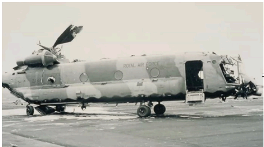
RAF Chinook helicopter – RAF Odiham (Almost certainly after 1981 – no actual date). Incorrect fitment of thrust race during overhaul of rear gearbox caused loss of axial location of drive pinion as aircraft lifted off, permitting pinion to loose tooth engagement with meshing ring gear. Hence front and rear rotors became unsynchronised and blades collided causing disruption of latter and shedding of tip weights with complete separation of front gearbox. There was damage to the structure and engine components, but no fatalities occurred on board.
