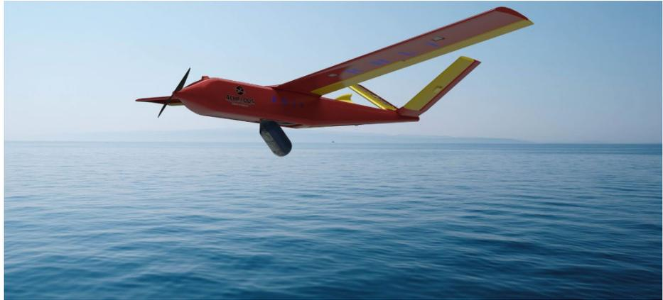
the search time. Refinement of searching algorithms alongside the camera systems allows for nearly 5 square nautical miles per hour to be searched when looking for a person in the water. Designed to provide the most effective assistance with a minimal burden on present practices. Achelous will be invaluable in helping the RNLI save lives from the skies.
